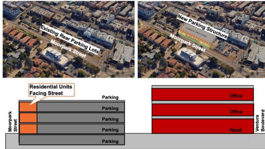
Figure 7. Parking Structures Could Be Built in Existing Parking-Zone Areas and Layered with Attractive Street-Facing Facades
