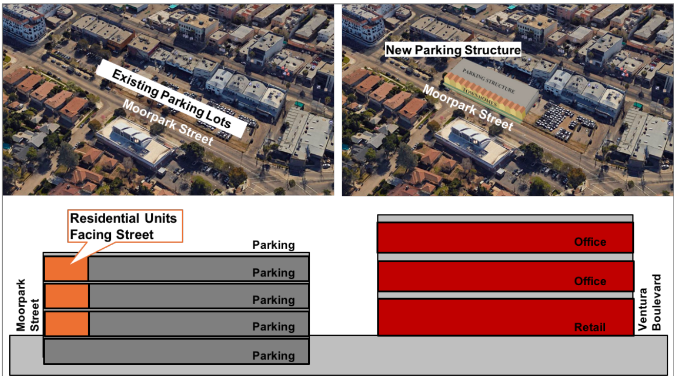
Figure 8. Parking Structures Could Be Built in Existing Parking-Zone Areas and Layered with Multifamily or Multiuse Buildings
